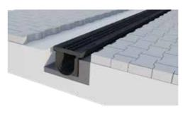
**8. Final Adjustments:** Ensure the grating is 3-5mm below the finished surface to complete the installation.
