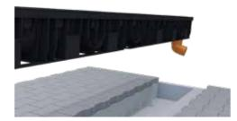
2. Trench Excavation: Ensure the trench is deep and wide enough to accommodate both the channel and bedding material. Keep the trench level and free of debris.
