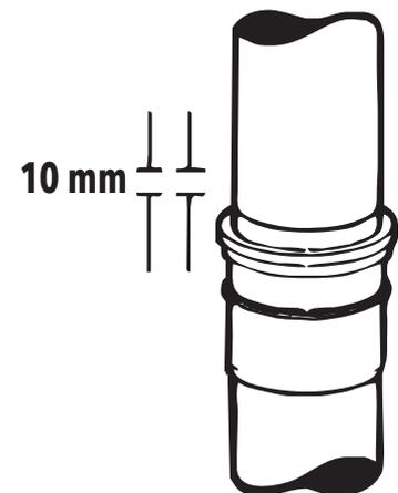
WITHDRAW PIPE (10 MM). THIS WILL ALLOW FOR EXPANSION. ALL FITTINGS MUST BE SUPPORTED BY A BRACKET WHEN INSTALLED VERTICALLY.
