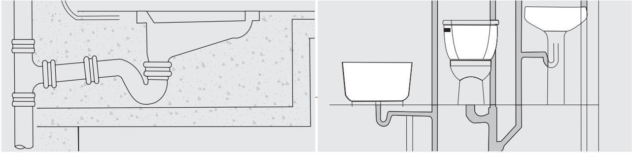
Traps are very important parts of drainage and sewage system and are most critical to ensure efficient working of the system. Traps prevent foul gases or air to enter back in passage and at a same time allow waste to flow through them.
